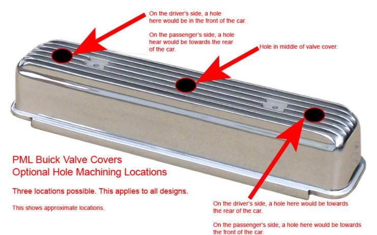
PML machines the holes to a diameter of 1<sup>1</sup>/<sub>4</sub> inches. The holes are spot faced for a good seal with the grommet. For oil fill, most folks remove the PCV or breather and fill there. PML can also drill and tap for an oil cap.
