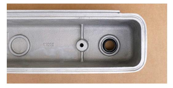
Holes machined on end toward the rear of the engine on both valve covers:
