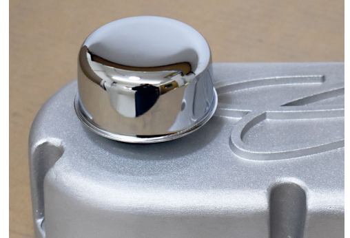
Raised CADILLAC script, Part Number 7872-8, As-Cast Finish, hole machined for breather grommet, breather grommet installed, breather cap installed. Note that this breather cap is large and overlaps the C in the script.
