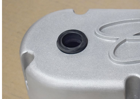
Raised CADILLAC script, Part Number 7872-8, As-Cast Finish, hole machined for breather grommet, breather grommet installed, breather cap installed. Note that this breather cap is large and overlaps the C in the script.
