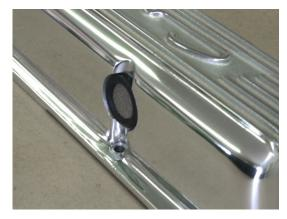
This is a close-up of a push-in breather installed in the hole on a PML valve cover.
