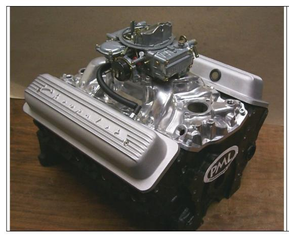
This picture shows a PCV valve plumbed to carburetor on the passenger's side and a baffled breather grommet shown installed on the driver's side.
