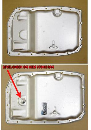
This document DOES NOT APPLY if the stock pan does NOT have a fill/level check at the rear of the pan. Example pictured at left. This is common with pre-2019 trucks and SUVs.
