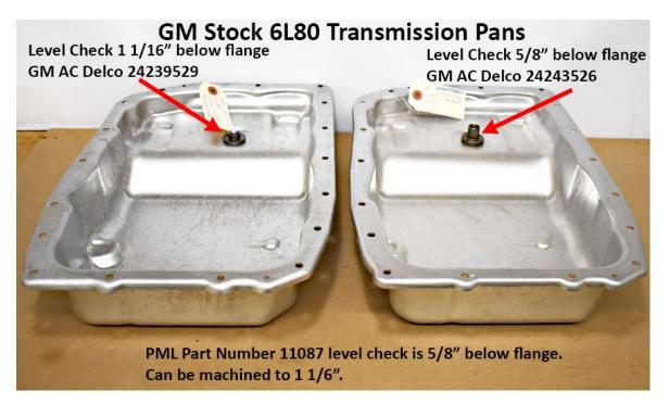
There could also be a problem with the PML pan hitting transmission internals if the heights do not match. So it is important to check the distance before installing.
