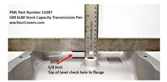
By default, this PML transmission pan has the level check is 5/8" below the flange. This can be machined to match the OEM pan. Call or email for information.
