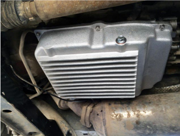
PML NAG1/722.6 installed.
