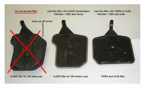
This pan is designed to work with the 4L60E and 700R4 filters that fit the GM shallow pans. These filters are seen above in the middle and on the right.
