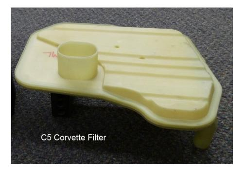
This filter has an extension at the inlet that will draw oil from deeper in the pan. Do not use regular 4L60E filters with the 8650-3 pan, only the C5 style.
