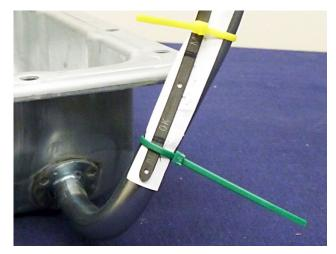
So with a PML AW4/A340 pan you do NOT use a dipstick. The OK and MAX fluid level checks are holes on the pan. Plugs for the holes are included.
