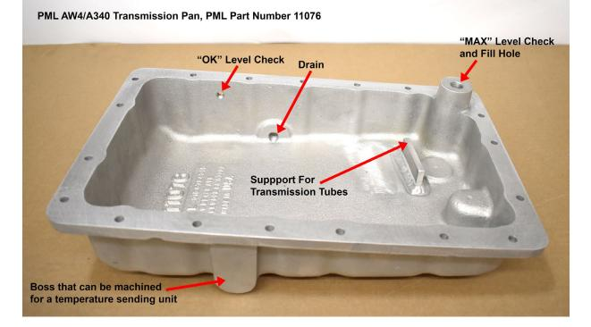
Once installed, the bottom of the transmission pan should be parallel to the ground for the fluid level check system on the PML pan to be accurate.
