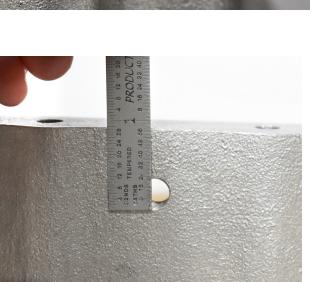
In addition to these rough manual measurements, PML laser scanned the parts and used computeraided design software to determine the locations. There is some variability since there is a big range between OK and MAX levels and the transmission housing flange is not parallel to the ground.
