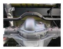
The axle is rotated as shown in this picture of a 2009 Wrangler. A PML cover will not work for these applications.
